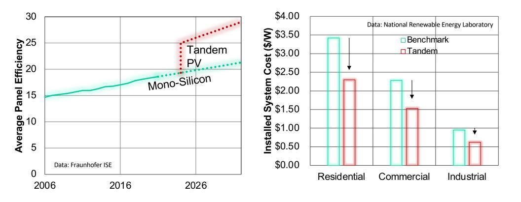
Step up in solar panel efficiency with tandems, otherwise 25% Silicon reached by line of sight only in 2050
